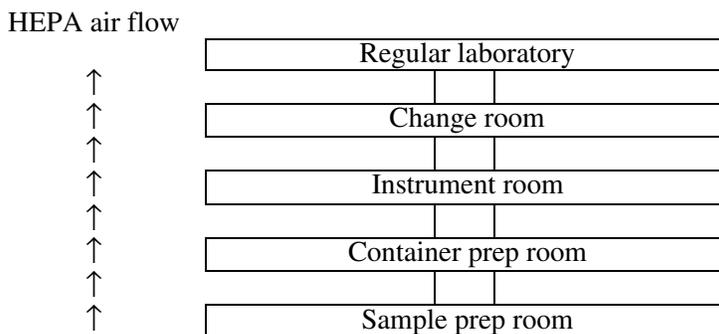
**Figure 9-1. Schematic of trace metals clean room facility.**
