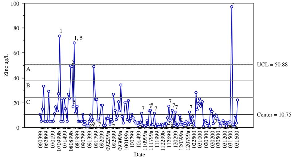
**Figure 9-2. Control chart for zinc preparation blanks by EPA Method 200.7.**
